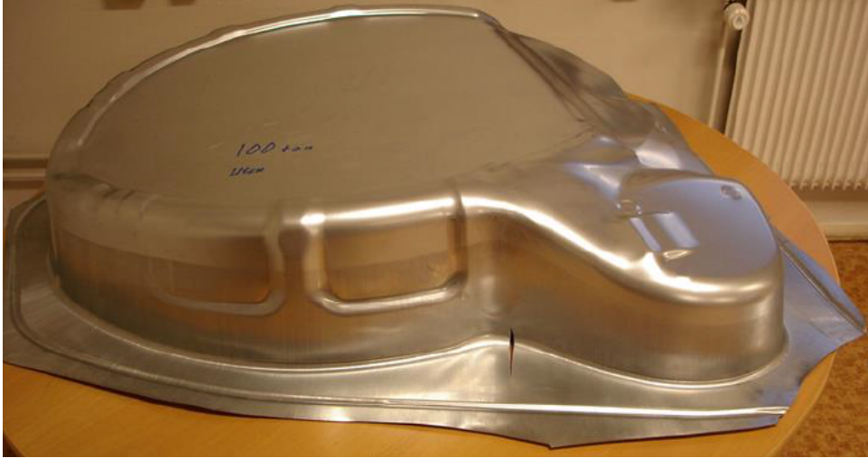
Fig. 1: Volvo Cars component showing failure due to Non-Linear Strain Path.
