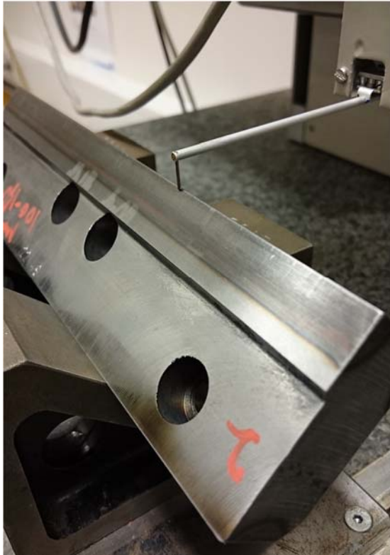
Figure 3.12. The Surfscan probe during measurement of worn cut tool.
