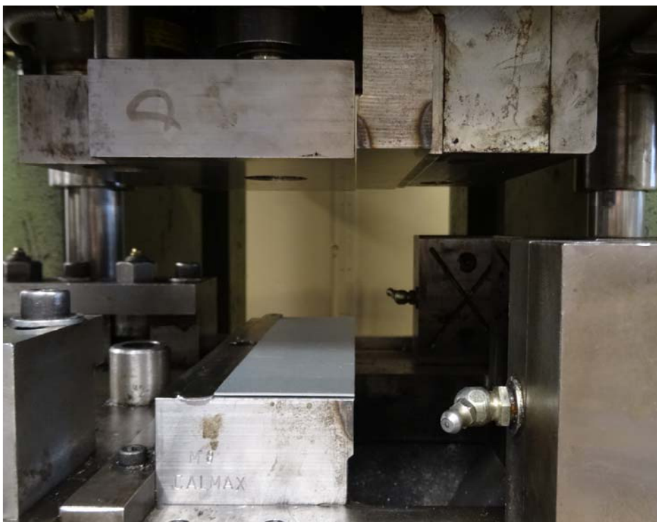
Figure 3.8. A finished test specimen after cut procedure.
