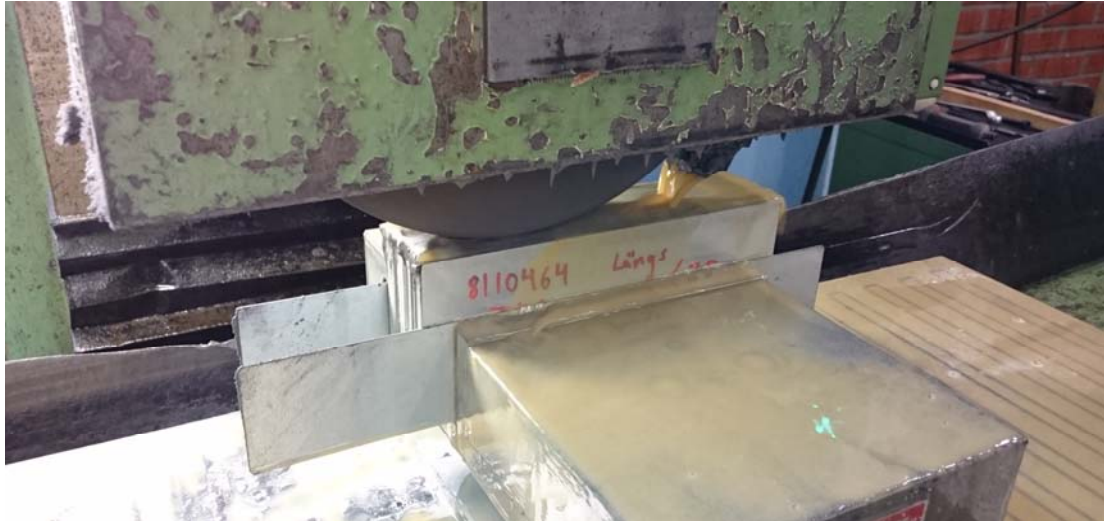
Figure 3.6. The polished edge of all specimens was prepared in an automatic grinding machine.
