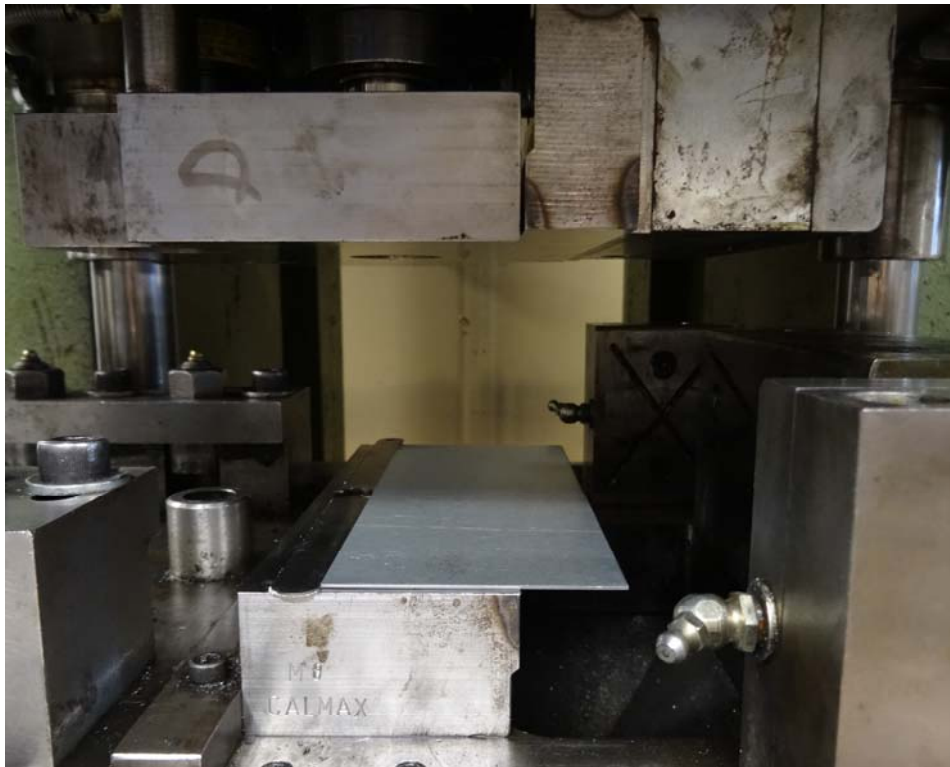
Figure 3.7. A test specimen before cut procedure.
