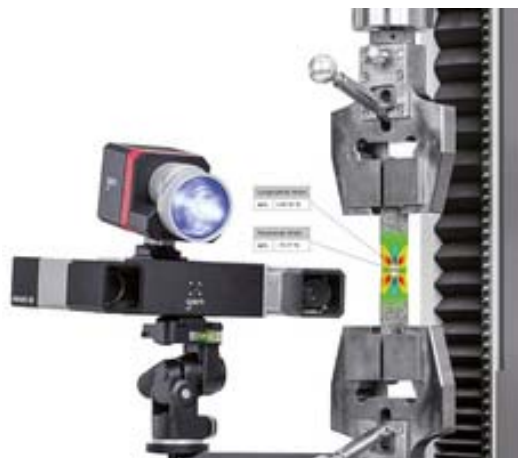
Figure 2.11. The two cameras of the ARAMIS system determine changes of the test specimen during a tensile test or similar tests [12].
