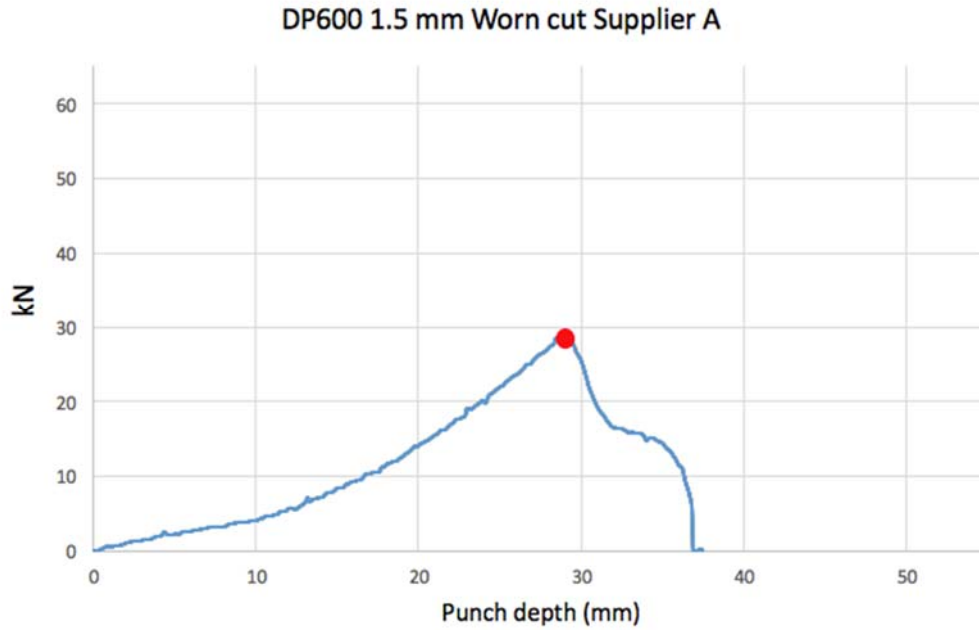
Diagram 4.12. The point where maximum force and punch depth is reached. Small fractures have already appeared at the sheared cut edge in this point and one of them will grow bigger and separate the specimen. This phenomenon was only seen from the results in ARAMIS.
