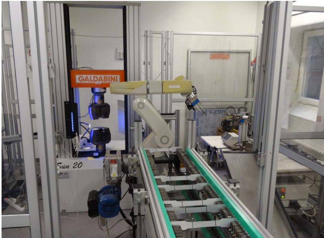
Figure 3.2. The automatic tensile test machine used for the tensile tests. Dog bone specimens ready for testing can be seen down in the middle.
