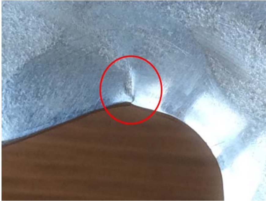
Figure 1.1. A fracture in a shear cut edge of a DP steel body part.
