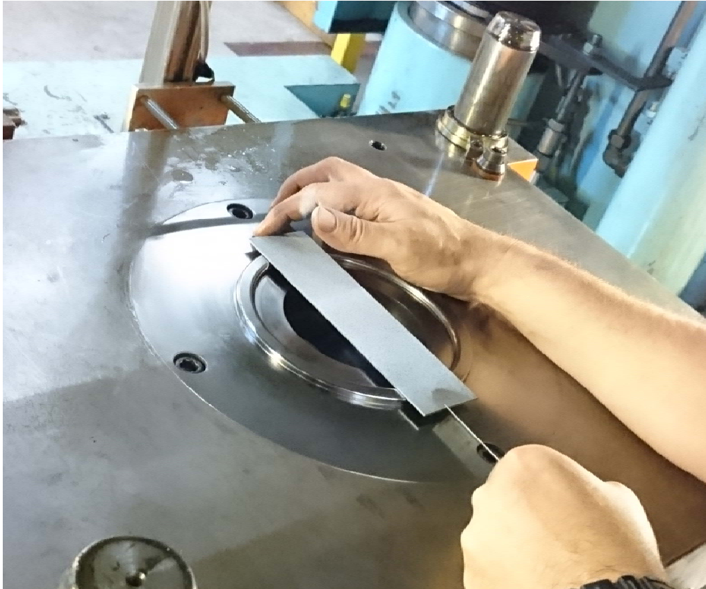
Figure 3.15. The painted test specimen was placed in the press and later formed until the maximum tensile strain was exceeded. The same test method was used for the experimental tests.
