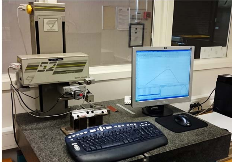
Figure 2.12. The Surfscan measurement system used for measurement of edge geometry in this study.
