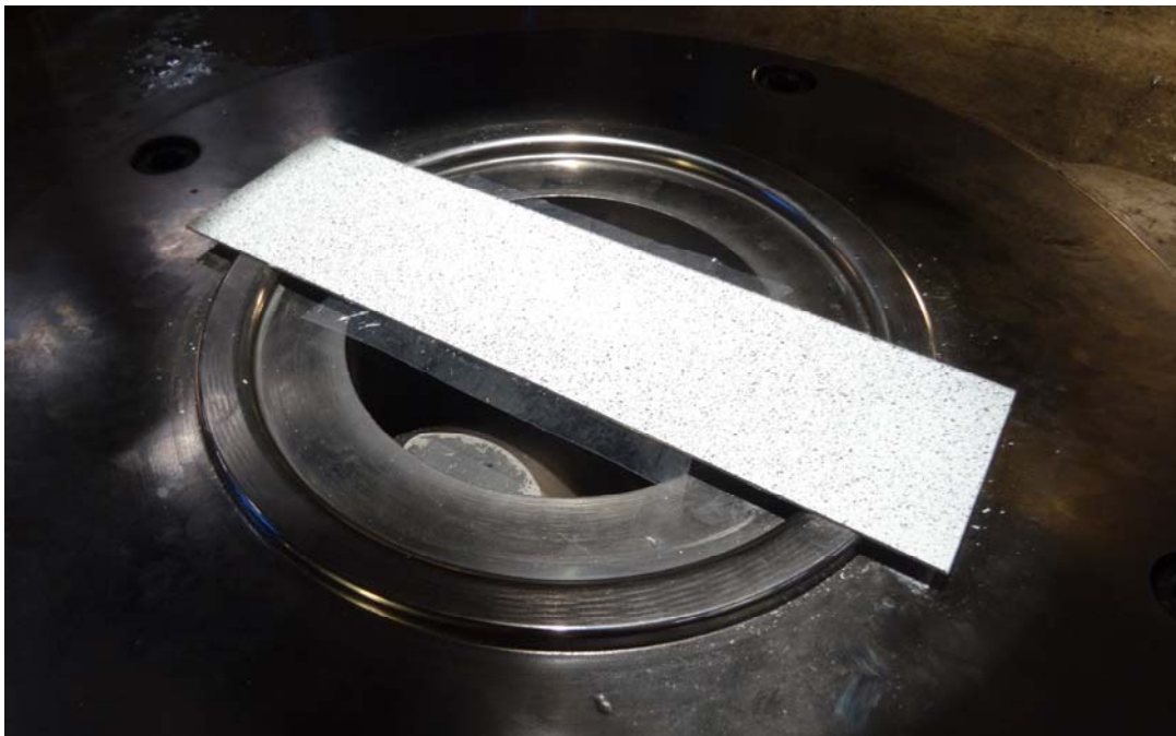
Figure 3.16. A specimen before the press operation.
