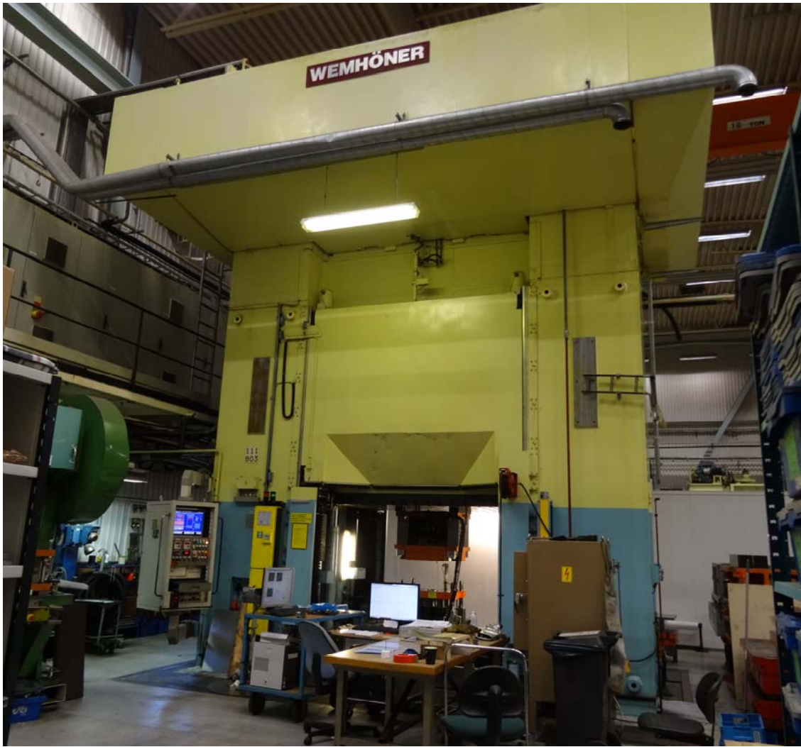
Figure 3.18. The press used for all tests. The two computers used for measuring can be seen in front of the press. One computer was used to measure forces and punch depth and the other computer was used for the ARAMIS DIC system.
