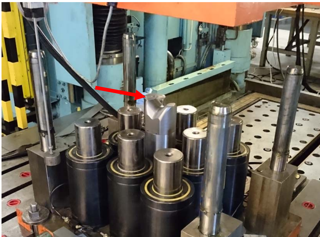
Figure 3.14. Installation of the CTEST punch in the press.
